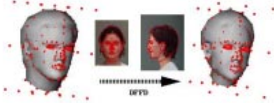
Figure 1: Modification of a generic head according to feature points detected on pictures. Points on a 3D head are control points for DFFD.
